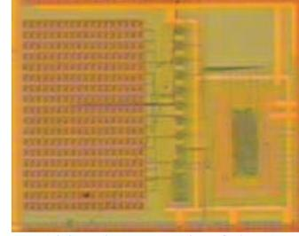
Figure 4. Chip photograph of the SAR ADC
