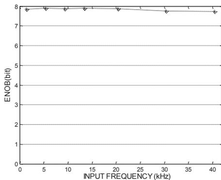
Figure 7. Measured ENOB versus different input sinusoidal frequencies
