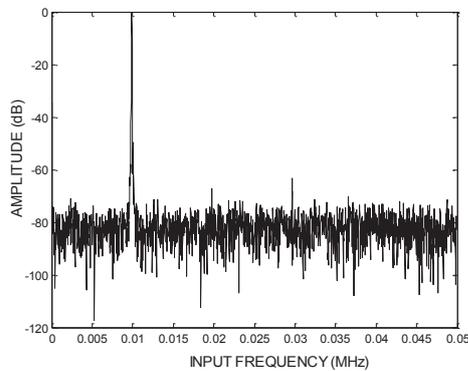
Figure 6. Measured output spectrum of SAR ADC with full-scale 9.37 kHz sinusoidal input waveform
