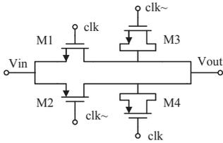
Figure 2. Complementary sampling switch S0 with dummy MOSFETs
