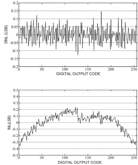
Figure 5. Measured DNL and INL plots of the SAR ADC
