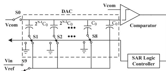
Figure 1. Architecture of proposed SAR ADC
